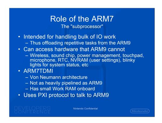
ARM7TDMI is the same kind of chip used in the GBA; makes sense given the GBA-compatible mode that DS has.
